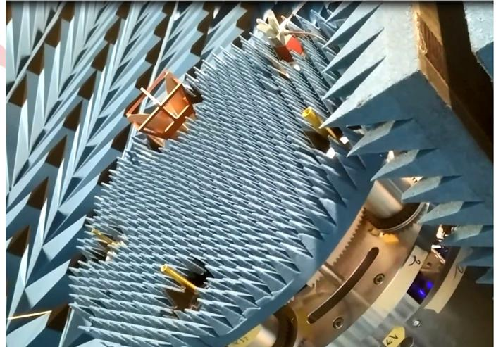
With full support for chapters 6 and 7 of 3GPP TS 38.141, the novel antenna feed carousel brings automation to an unheard-of level in gNodeB OTA testing. Several RF paths with different signal levels, in combination to mmWave oscillators, switches, amplifiers, multipliers, mixers and combiners, set the pace for world-wide first OTA tests up to 220 GHz with the push of a button. The system is currently in use at two customer sites, leading manufacturers of gNodeB.
